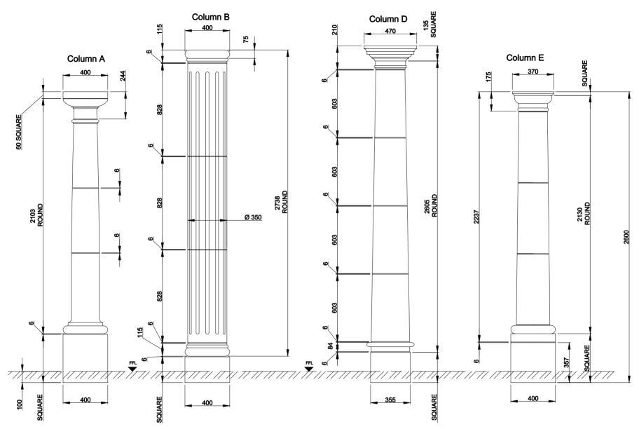
HEIGHT VARIATIONS ARE OBTAINED BY INCREASING THE BASE BLOCK HEIGHT. COLUMNS SUPPLIED SOLID OR IN HOLLOW SECTION (SOME COLUMNS ARE NOT AVAILABLE WITH HOLLOW OPTION).
